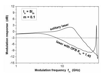
FIG. 1 Numerical modulation responses of both the solitary laser and laser under strong OFB  $K_{ex}$  = 1.45, when  $I_b$  = 5 $I_{th}$  and m = 0.1.
