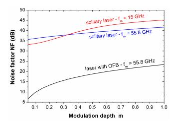
FIG. 5 Noise factor as a function of modulation depth m of the laser under OFB when modulated with  $f_m$  = 55.8 GHz and the solitary laser when modulated with  $f_m$  = 15 and 55.8 GHz.
