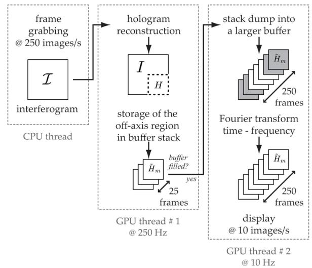
FIG. 2 Algorithmic layout of holographic rendering. Raw interferograms are recorded by the main CPU thread. Spatial Fresnel transforms are performed by the first GPU thread. Short-time temporal Fourier transforms are performed by the second GPU thread.
