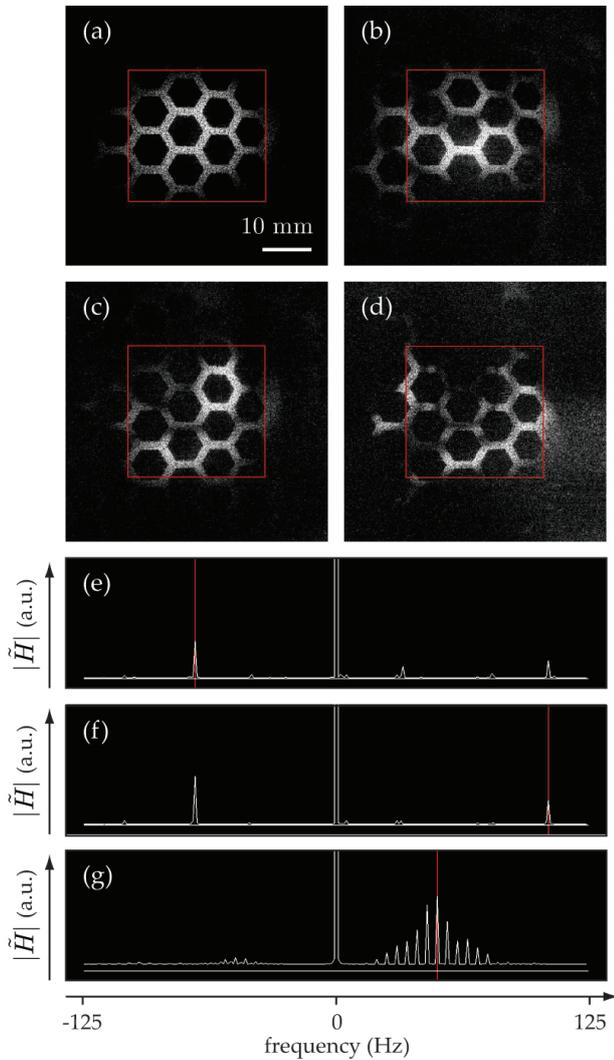
FIG. 4 Short-time Fourier transform vibration maps and spectra of a metal structure excited sinusoidally. No excitation (a). Excitation at  $P = 2$  frequencies:  $\nu_{M_1} = 3200 + 100$  Hz and  $\nu_{M_2} = 3200 - 70$  Hz (b-c,e-f). Excitation at  $P = 2$  frequencies:  $\nu_{M_1} = 3200 + 50$  Hz and  $\nu_{M_2} = 3200 + 45$  Hz (d,g). LO detuning:  $\Delta\nu = 3200$  Hz; The movie of the experiment is reported in media 1 (videofile: 9.1 MB, format: avi, see Movie)
