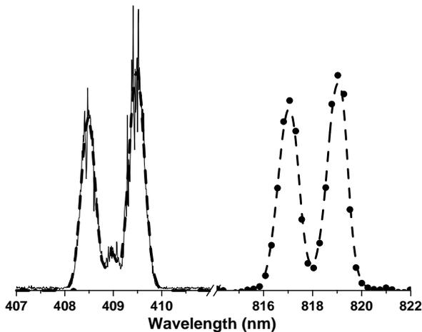
FIG. 7 (Right) Dual wavelength lasing (816.96 and 818.97 nm,  $\Delta\nu = 0.901$  THz) and (Left) signal through a BBO crystal producing SHG (408.48 and 409.48 nm) and SFG (408.96 nm). The relative height of the converted peaks are: 1.00 (408.48 nm), 0.28 (408.96 nm), and 1.25 (409.48 nm).
