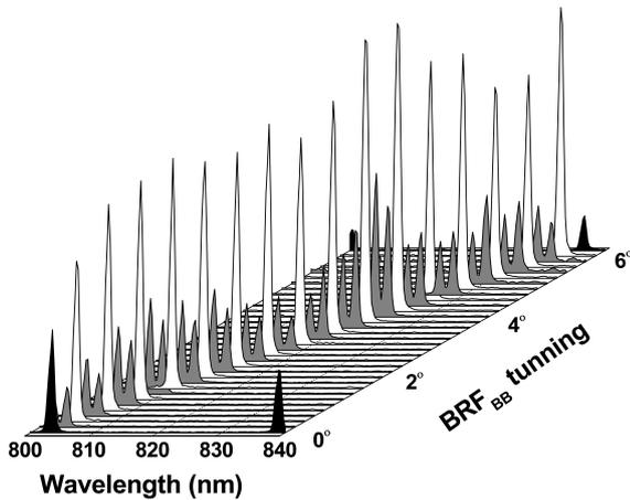
FIG. 6 Laser tuning as function of  $BRF_{BB}$  rotation with both  $BRF_{BB}$  and  $BRF_{DW}$  in the cavity. The laser switches between single wavelength operation (white spectra) and double wavelength operation (grey spectra) within the FSR range of the  $BRF_{BB}$  (black spectra).
