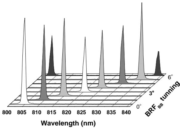
FIG. 3 Laser tuning with only the  $BRF_{BB}$  plate in the cavity. Notice the dual wavelength operation at the edge of the tuning range (black spectra).
