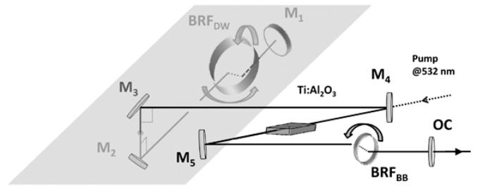
FIG. 2 Dual wavelength laser setup based on a Ti:Al<sub>2</sub>O<sub>3</sub> crystal. M<sub>1</sub> to M<sub>5</sub> are dielectric IR mirrors, M<sub>4</sub> is a dichroic mirror. OC: Output Coupler. M<sub>2</sub> and M<sub>3</sub> form a 90° periscope. BRF<sub>BB</sub> is the narrow broadband filter and BRF<sub>DW</sub> is the thick filter as described in the text.
