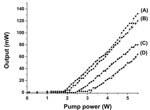
FIG. 5 Laser emission characteristic at 814.6 nm for (A) cavity without BRF, (B) with only  $BRF_{BB}$  in the cavity; (C) with  $BRF_{BB}$  and  $BRF_{DW}$  in the cavity in single wavelength operation and (D)  $BRF_{BB}$  and  $BRF_{DW}$  in the cavity in dual wavelength operation.
