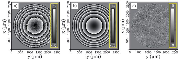
FIG. 9 Comparison between the phase distributions of the test lens obtained from the experiment and simulation: (a) Filtered version of the retrieved phase distribution of the thin lens shown by Figure 8. (b) Numerical simulation of the test lens refractive profile. (c) Subtraction of the two phase distributions.
