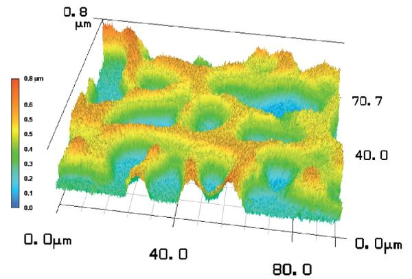
FIG. 2 Three-dimensional height map of the fabricated RPD plate for a cross-section of  $95 \times 65 \mu\text{m}^2$  measured by Keyence microscope.
