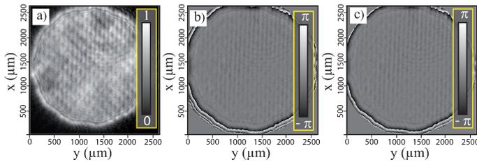
FIG. 5 Experimental results for setup without phase diffuser: (a) Observed real amplitude in the sensor domain. Phase recovered after 200 iterations for a plane wave that is incident (b) parallel to and (c) at an angle with respect to the optical axis of the setup. (All distributions: 750 x 750 pixels with a pixel pitch of 3.45  $\mu\text{m}$ ).
