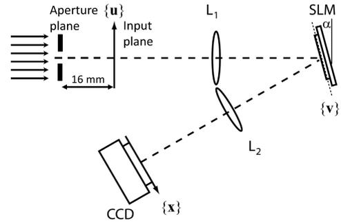
FIG. 4 A plane wave is incident on an aperture (without diffuser phase plate) and the transmitted light is directed to SLM-PR setup.  $\alpha$  is a small tilt angle,  $u$ ,  $x$  and  $v$  are the coordinates at the input, the camera and the common Fourier planes, respectively.  $L_1$  and  $L_2$  denote two identical lenses and SLM refers to the spatial light modulator.
