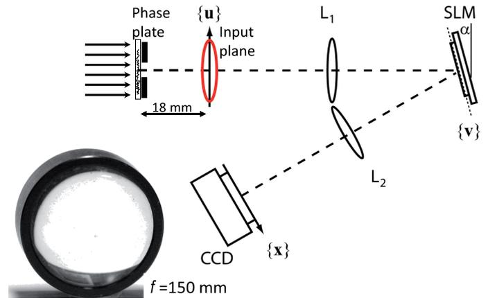
FIG. 7 The scheme of the SLM-PR setup used to determine the phase variation of a plane wave after its modulation with a thin lens having a focal length of  $f = 150$  mm.
