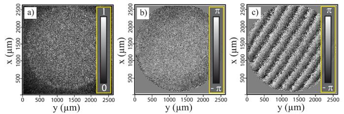
FIG. 6 Experimental results obtained after introducing the desired diversity by means of the fabricated RPD plate: (a) Observed real amplitude in the sensor domain. Phase recovered after 200 iterations for a plane wave that is incident parallel to (b) and, at an angle with respect to the optical axis of the setup (c). (All distributions: 750 x 750 pixels with a pixel pitch of 3.45  $\mu\text{m}$ ).
