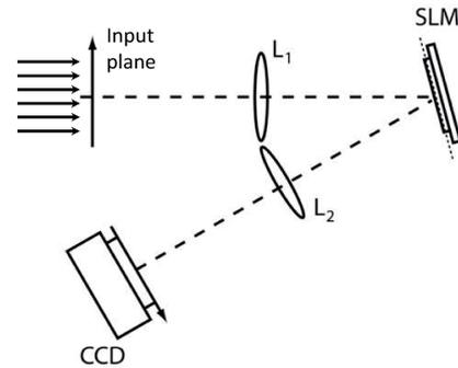
FIG. 1 Sketch of the SLM-PR setup. SLM refers to a phase-only spatial light modulator, CCD or charge-coupled device is the recording camera and  $L_1$  and  $L_2$  are identical lenses.
