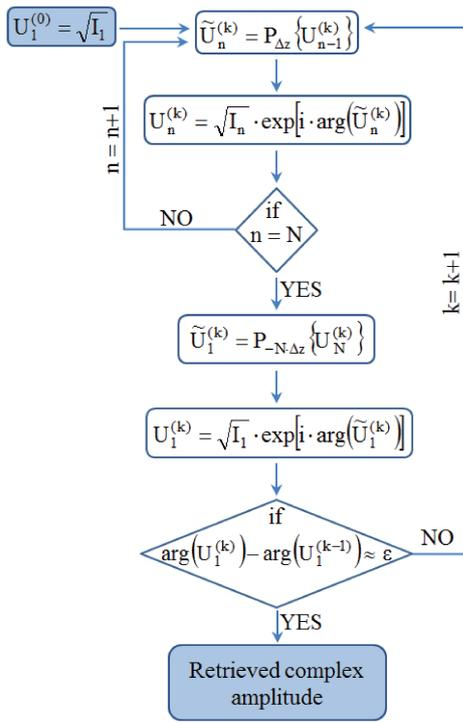
FIG. 3 Flowchart of the iterative phase retrieval, where  $n$  represents the propagation plane number and it varies from 1 to  $N$ ,  $k$  stands for the iteration number and  $\tilde{U}$  and  $U$  denote the resulting complex amplitudes directly after applying the propagation operator and after exchanging the real amplitude with the square root of the measured intensity.
