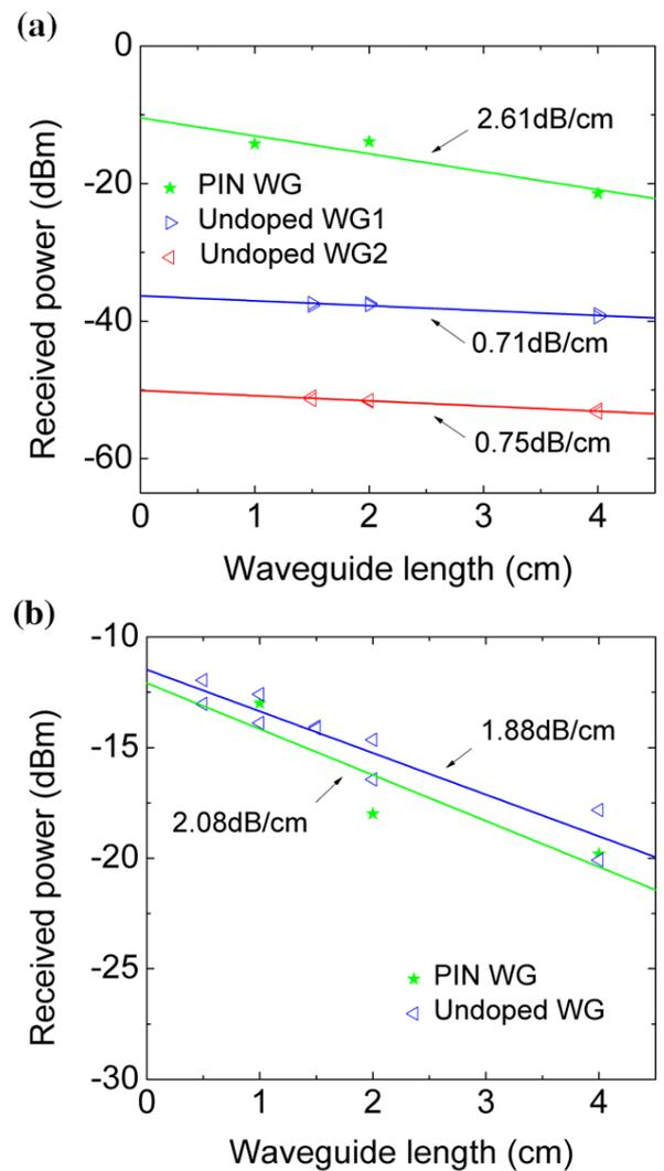
FIG. 5 Cut-back measurement results for (a) shallow etched waveguides and (b) deep etched waveguides. The green symbols represent TE-transmission signals for waveguides with embedded PIN and the slopes of the fitting lines show the losses for (a) shallow etched waveguides and (b) deep etched waveguides, 2.61 dB/cm and 2.08 dB/cm, respectively. The blue and red symbols represent the measurement results for undoped waveguides. The losses are indicated in the figures.
