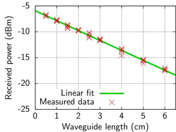
FIG. 1 Cut-back measurement results for 450 nm waveguides. Each symbol represents a TE-transmission signal through a waveguide with a certain length. The solid line is the linear fit showing a loss of 1.7 dB/cm.
