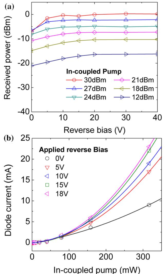
FIG. 6 Experimental results from the deep-etched E/O waveguide of 4 cm length. (a) Received power versus applied reverse bias voltage for different in-coupled pump power. Power values were measured by optical spectrum analyzer and therefore attenuated by 14 dB. (b) Diode current as a function of the in-coupled pump in the waveguide for different applied reverse bias. Symbols represent the experimental data and solid curves are the quadratic fits.
