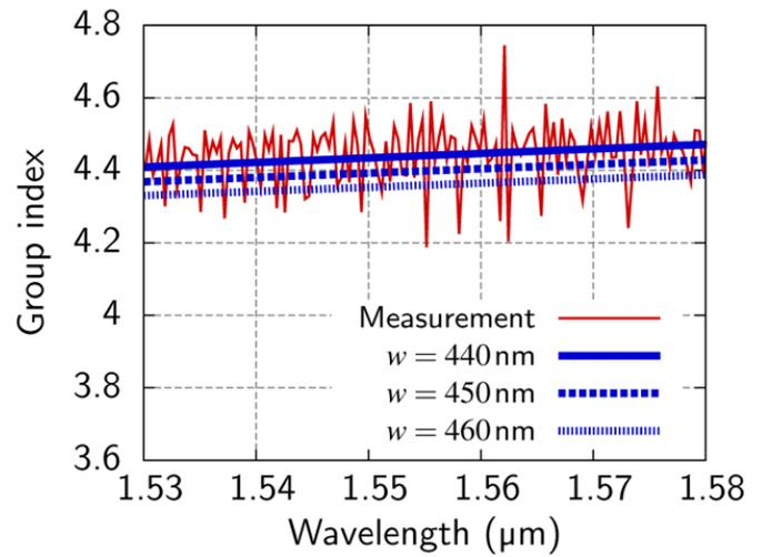
FIG. 3 Measurement and simulation results of group index dependence on wavelength in C-band for standard waveguide. The dashed lines represent numerical results for waveguides of varying width (440 nm, 450 nm and 460 nm).
