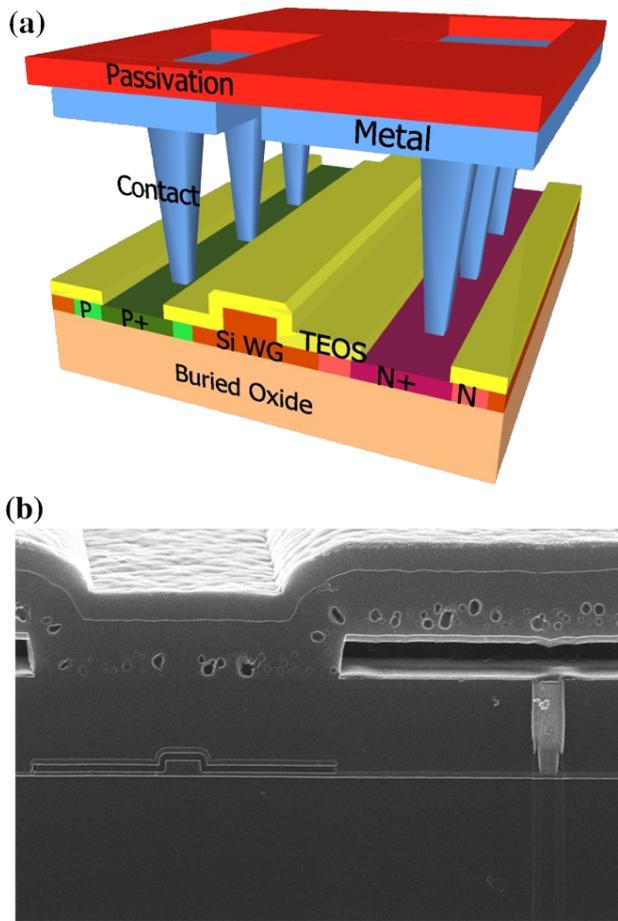
FIG. 4 (a) Schematic geometry of the E/O waveguide. (b) FIB image of the cross section.
