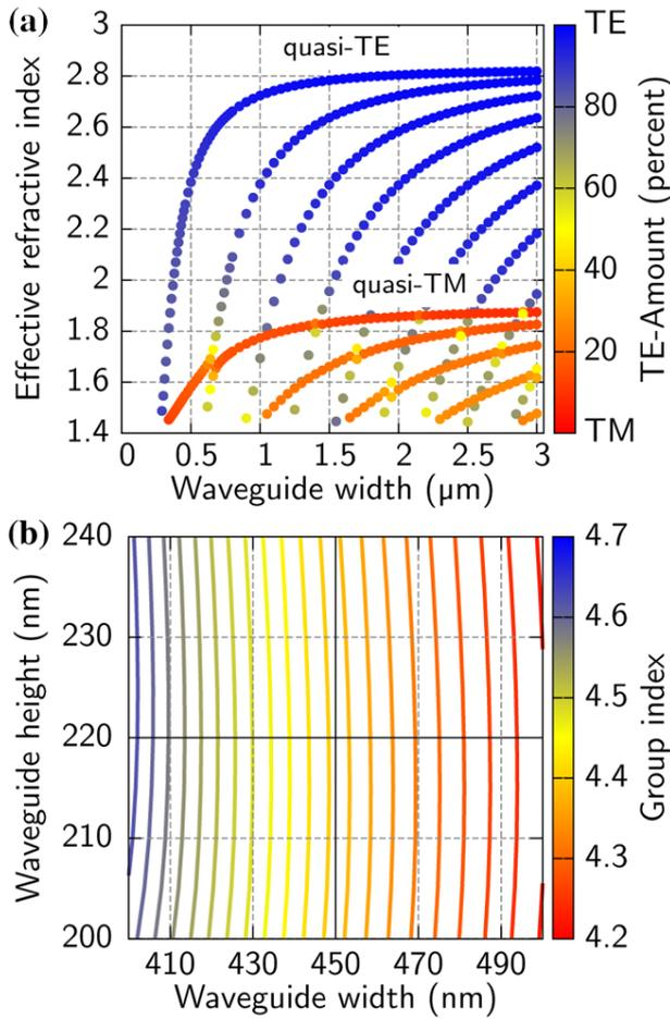
FIG. 2 (a) Numerical effective indices for the first guided modes in nano-strip waveguides as a function of waveguide width. The color indicates hybridness of the mode. (b) Numerical group index versus the waveguide geometry for the fundamental quasi-TE mode around the standard dimensions (450 nm x 220 nm). The contour lines represent waveguide geometries of constant group index.
