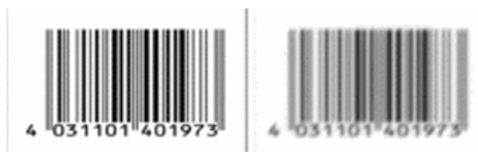
FIG. 1 left: image definition without safety glasses, right: image definition with safety glasses, DIN EN 166 conform (simulation)
