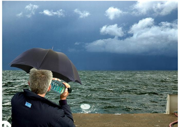
FIG. 4 A FU observation is taken, at the shady side of the vessel, above a submersed Secchi disc, with the disc lowered to a depth of approximately half the Secchi disc depth. The reading of the scale should be done in the shadow.
