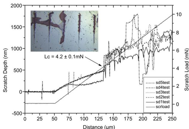
FIG. 4 Comparison of Scratch tests curves on a-Si:H side (with optical image in the plot inset)
