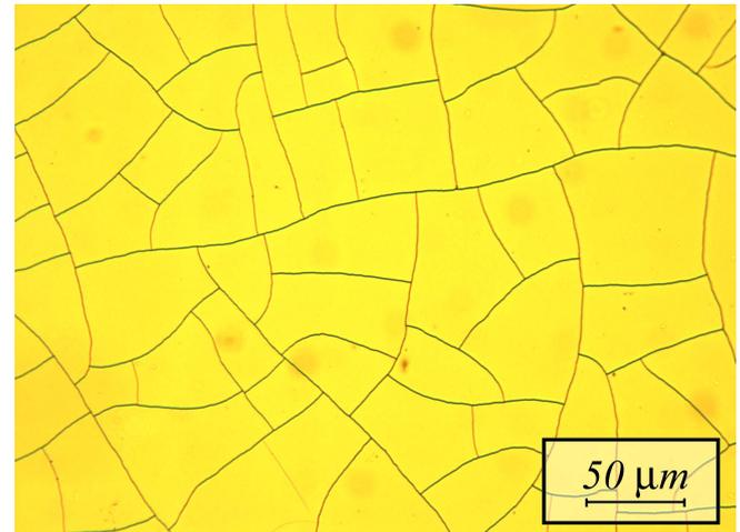
FIG. 3 Optical microscopy of a-Si:H film deposited as top layer. Magnification of 20×
