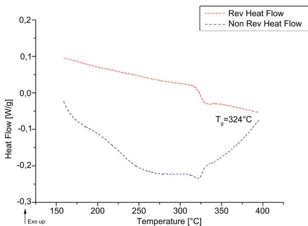
FIG. 2 Modulated Differential Scanning Calorimetry of AryLite™
