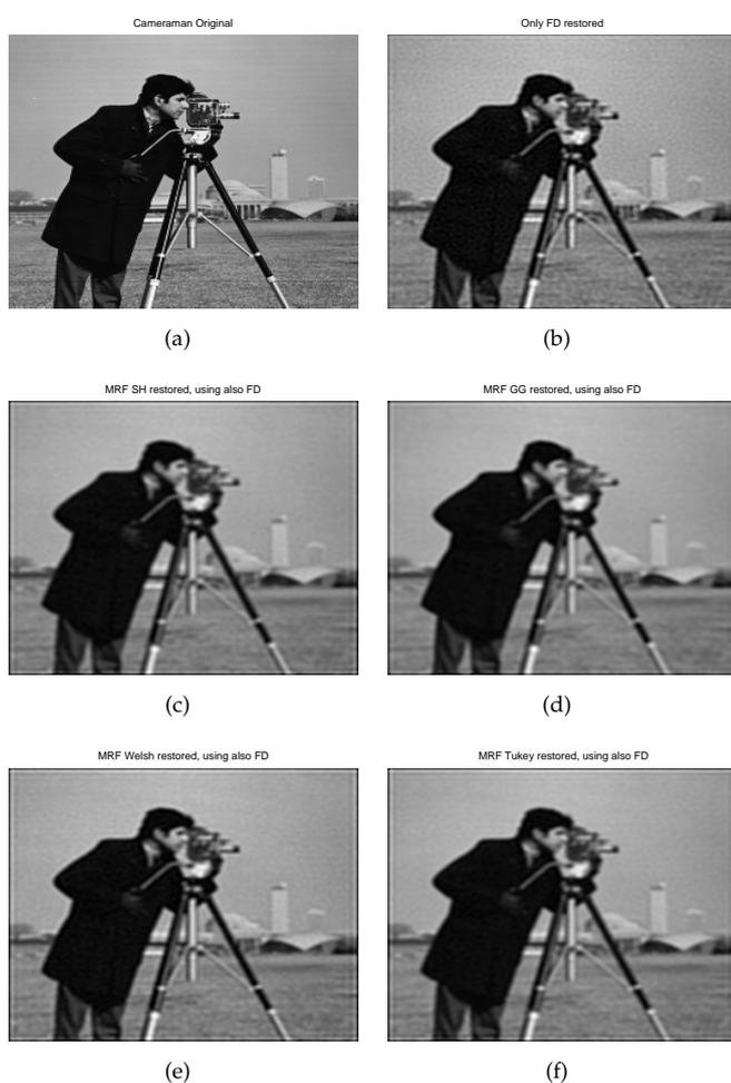
FIG. 8 Results for Cameraman standard image: (a) describes the original image; (b) describes restored image using only a frequency domain (FD) deconvolution technique; (c) restored image using MAP2 and FD ( $\Delta_0 = 20$ ); (d) restored image using MAP1 and FD ( $\lambda = 0.15, p = 1.2$ ); (e) restored image using MAP3 and FD ( $k_g = 2000, \mu = 0.0015, \lambda = 10$ ); (f) restored image using MAP4 and FD ( $k_g = 2000, \mu = 0.0015, \lambda = 10$ ).
