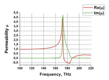
FIG. 6 Retrieved permeability spectrum of the SCube structure
