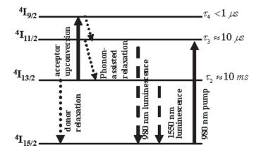
FIG. 1 Erbium ion transition diagram. Upconversion process on metastable  $({}^{4}l_{13/2})$  level: the donor ion is deactivated whereas the acceptor is exited to  ${}^{4}l_{9/2}$  level. Relaxation of  ${}^{4}l_{9/2}$  level: non-radiative phonon-assisted, and radiative relaxation from the second exited level  $({}^{4}l_{11/2})$  result in 980 nm fluorescence. Radiative relaxation from the metastable level causes 1550 nm fluorescence.
