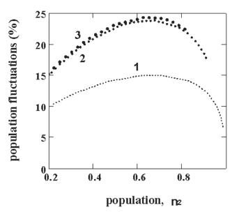
FIG. 2 Population fluctuations  $\delta$  as a function of population of the first excited state  $n_2$  and normalised concentration of erbium ions  $\gamma$ . Parameters: r = 60,  $\beta = 1$  (pump at 980 nm [6]),  $\gamma = 0.1$  (1),  $\gamma = 1$  (2),  $\gamma = 2$  (3).
