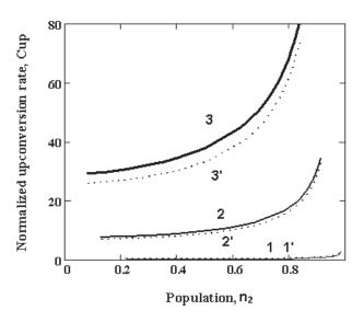
FIG. 3 Normalised upconversion coefficient  $C_{up}$  as a function of population of the first excited state  $n_2$  and normalised concentration of erbium ions  $\gamma$ . Parameters: r = 60,  $\beta = 1$  (pump at 980 nm [6]),  $\gamma = 0.1$  (1, 1'),  $\gamma = 1$  (2, 2'),  $\gamma = 2$  (3, 3'). Simplified model (Eqs. (2) and (11):  $\langle \sigma_m^2 \rangle = 0$ ) [5] (solid lines), generalised model (Eqs. (2) and (18):  $\langle \sigma_m^2 \rangle \neq 0$ ) (dotted lines).
