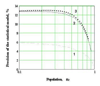
FIG. 4 Precision of the statistical model of upconversion *epsilon* as a function of population of the first excited state  $n_2$  and normalised concentration of erbium ions  $\gamma$ . Parameters: r = 60,  $\beta = 1$  (pump at 980 nm [6]),  $\gamma = 0.1$  (1),  $\gamma = 1$  (2),  $\gamma = 2$  (3).
